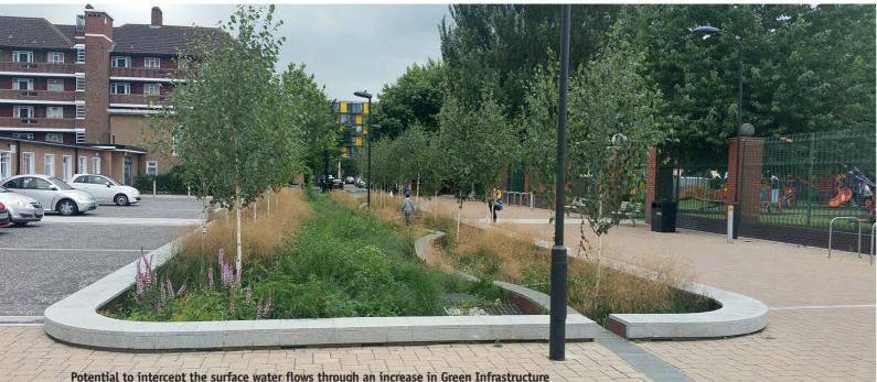
Potential to intercept the surface water flows through an increase in Green Infrastructure whilst putting place at heart of the design. (Image Courtesy of susdrain)
