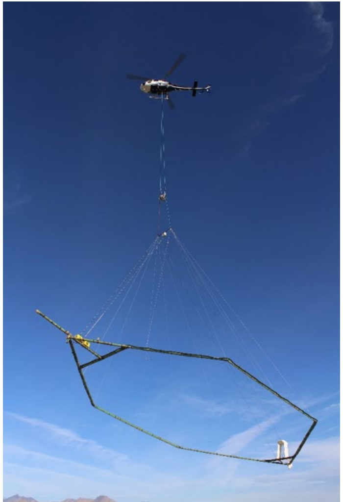
The SkyTEM AEM system during takeoff in Indian Wells Valley, California. SkyTEM is a geophysical survey company involved in implementing AEM surveys. Source: Ramboll Project File.
